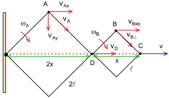
$$v = \frac{3x}{t} \quad v_D = \frac{2x}{t} = \frac{2v}{3} \quad v_{Ax} = \frac{x}{t} = \frac{v}{3} \quad v_{Bx} = \frac{5x}{2t} = \frac{5}{2} \frac{v}{3} = \frac{5v}{6} \quad v_{Bx_b} = v_{Bx} - v_D = \frac{5v}{6} - \frac{2v}{3} = \frac{v}{6}$$
