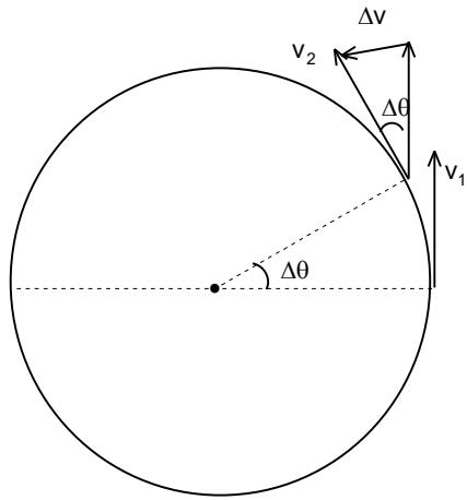
$$\frac{\Delta v}{\Delta t} = \frac{v \Delta \theta}{\Delta t} = v \frac{\Delta \theta}{\Delta t} = v \frac{\frac{v \Delta t}{r}}{\Delta t} = \frac{v^2}{r}$$
